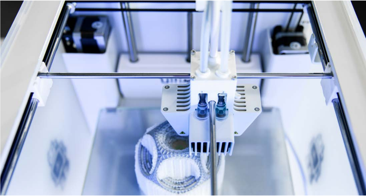
A PLA and PVA dual extrusion print. The white PVA material supports the part during printing, then can be dissolved away in water
